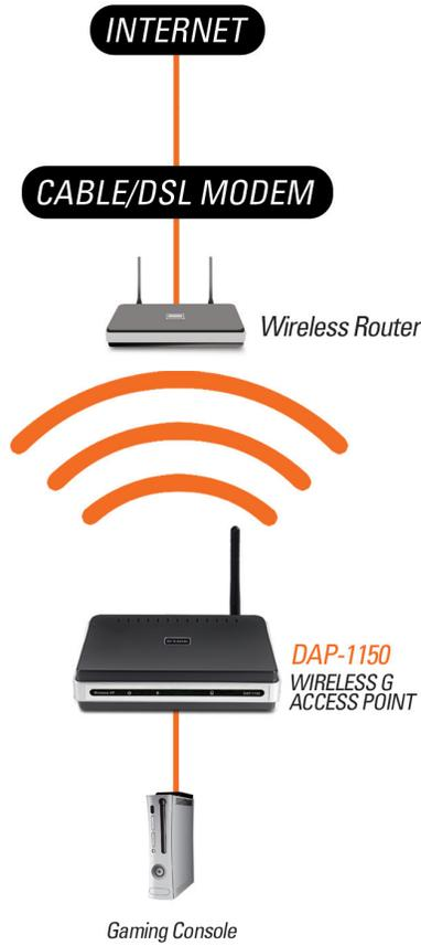
Connect an Ethernet-enabled gaming console to the Internet by using the DAP-1150 as a wireless interface
