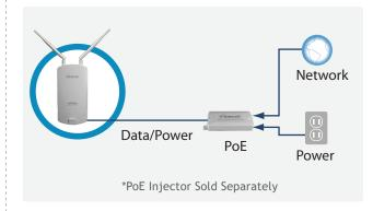
By combining your power and data connections into a single cable, PoE can simplify the setup. This gives you flexibility to install the device in any location, even out of the way locations with few power outlets.
