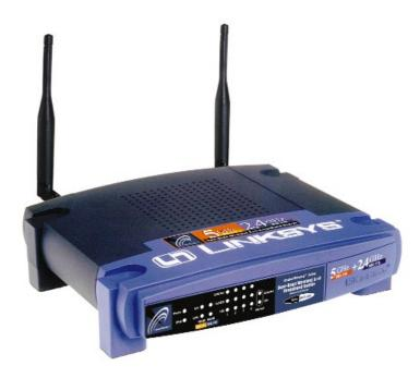
Dual-Band Wireless A+B Broadband Router Model No.: WRT51AB
