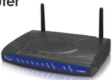
The CT-5364A Wireless Router provides wired and wireless access for high-bandwidth applications at home or in the office. It includes one ADSL2/2+ port, four Ethernet LAN ports, one Ethernet WAN port and an USB host port for printer support. An integrated 802.11n (2x2 MIMO) Access Point provides broadband wireless coverage (up to 270 Mbps) with backwards-compatibility for 802.11b/g and added WPS support.
