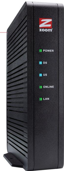
The Zoom Model 5370 cable modem meets the cable industry's DOCSIS 3.0 standard for speeds up to 686 Mbps, and also works with lower-speed DOCSIS 2.0 and 1.1 services. Full-Band Capture Digital Tuning allows service providers to offer more channels and accelerate downloads. The Model 5370 has been tested and certified by CableLabs® to work with nearly all U.S. cable services.
