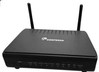
AR-5310u is an 802.11n (300Mbps) Wireless ADSL2+ router comprising four 10/100 Base-T Ethernet ports, a Wi-Fi Protected Setup (WPS)/ Wi-Fi switch button, a USB Host, and is backward compatible with existing 802.11b (11Mbps) and 11g (54bps) equipment.
