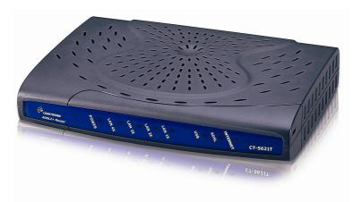
The CT-5621T ADSL2+ Multi-port Router has four Fast Ethernet ports and a single USB port for wired connectivity. It is designed for either home or business applications that require connectivity to an ADSL broadband network. The TR-068 compliant front and rear panels are a key feature which makes the CT-5621T easy to setup and use. Additionally, TR-069 compliance allows for auto configuration and remote management control via a remote ACS.
