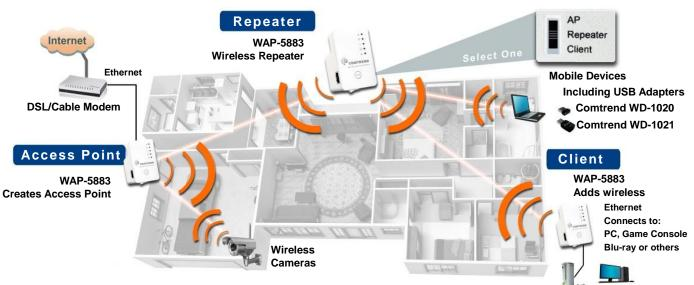
Repeater mode extends the wireless network for 802.11 (b/g/n) devices.
