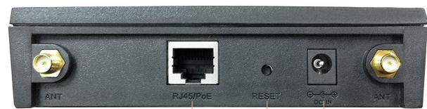
Ethernet port      Reset to default      Power DC inject
