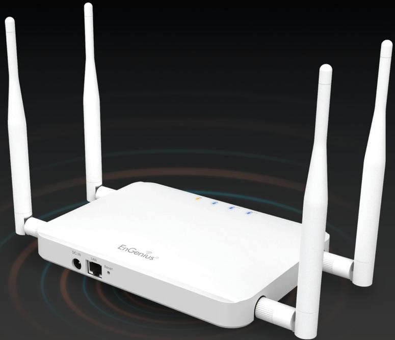
The EnGenius ECB600 is a concurrent dual band 2.4 / 5 GHz Wireless-N Indoor Access Point that features high transmit RF power (29 dBm on 2.4GHz and 26 dBm on 5GHz) for long range connectivity. With wireless speeds up to 300Mbps on each radio and a Gigabit port for connecting to a switch or router it's ideal for expanding a network with additional bandwidth to support additional users.
