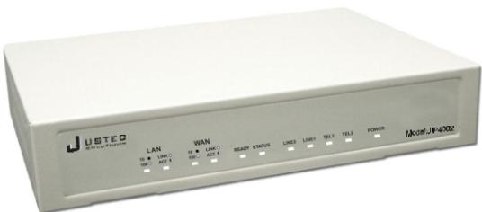
JIP4002 is a two-port FXS + FXO gateway and support H.323 v2/v3/v4 or SIP RFC 3261 protocol. It supports an innovative intelligent call routing function that transparently routes calls to destination either through PSTN or internet. JIP4002 provides Voice over IP and FAX over IP services for ITSP / ISP (Internet Telephony Services Provider) and Office / SOHO IP-PBX application.
