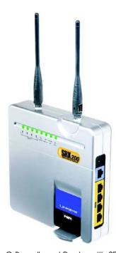
The Wireless-G Broadband Router with SRX200 is really three devices in one box. First, there's the Wireless Access Point, which lets you connect Wireless-G, Wireless-B, and other performance-enhanced SRX devices to the network. There's also a built-in 4-port full-duplex 10/100 Switch to connect your wired-Ethernet devices together. Finally, the Router function ties it all together and lets your whole network share a high-speed cable or DSL Internet connection.
