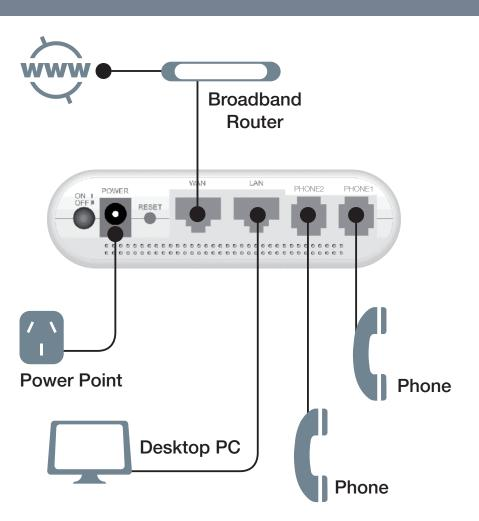
NetComm's V220 VoIP Telephone Adaptor has been designed for residential and small business users to deliver predictable real-time voice quality over the Internet. It connects directly to any broadband modem and service (Cable or DSL) plus an account with a VoIP Service Provider.
