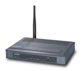
The PLANET WNAP-1110 is the 802.11n Wireless Access Point backward compatible with 802.11b/g and its transmitting data rate can be up to 150Mbps. The wireless AP features radio in 1x1 (TX / RX) of intelligent antennas offering high performance and superior coverage range.
