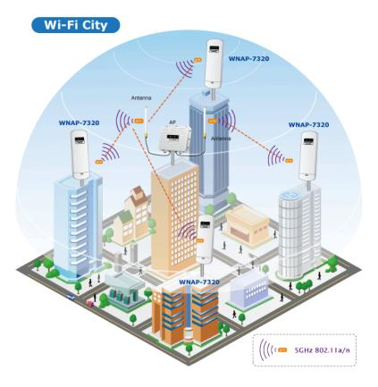
With built-in 14dBi dual-polarization directional antenna, the WNAP-7320 brings higher coverage and longer distance of wireless connection. The WNAP-7320 provides high output power with multiple adjust Tx controller, which allows CPE users to easily install and adjust the suitable value in appropriate locations. Moreover, the WNAP-7320 supports WISP mode to enable CPE users to connect to Internet via local WISP provider.
