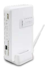
PLANET 3G Broadband Router, the WNRT-626G, provides Internet access via mobile network by CDMA2000 / UMTS / HSDPA protocol and 3G Internet USB card. It features 802.11n radio with 1T1R antenna technology and backward compliant with 802.11g and 802.11b standards. Compared with general wireless routers, the WNRT-626G offers more powerful and flexible capability for LAN clients to access Internet with management functions.
