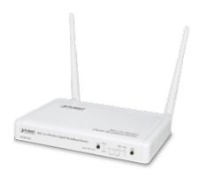
The PLANET WNRT-632 wireless Gigabit broadband router is a built-in 802.11n 2.0 access point (AP) and backward compatible with 802.11b/g. The wireless Gigabit router features radio in 2x2 (Tx/Rx) of intelligent antennas offering high performance and superior coverage range.
