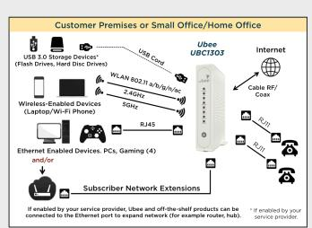
WI-FI Connectivity & Security - Provides dual-band concurrent 2.4GHz and 5GHz radios. 8 SSIDs per radio offer considerable flexibility for the customer's network. The residential gateway with an integrated 802.11ac access point gives users the flexibility to connect a variety of home and mobile devices. 4 transmit and 4 receive internal antennas enables high wireless
