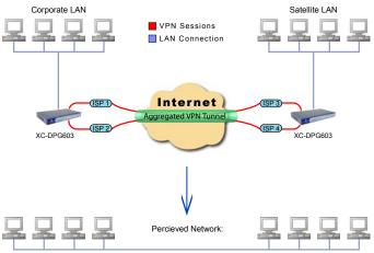
Aggregating traffic requests over two concurrent VPN tunnels provides increase bandwidth for a Virtual Private Network
