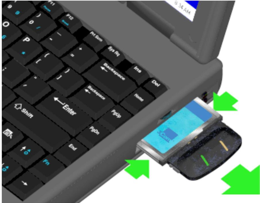
**CAUTION:** *The antenna on the PC Card is not removable. If you try to remove the card by pulling on the antenna, you may break the antenna and permanently damage the card.*
