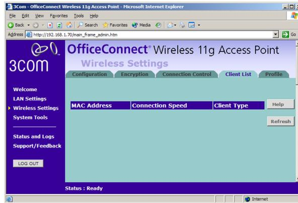
The Wireless Client List provides details on the devices that are connected to the Wireless LAN. The list is only created when Wireless Networking is enabled. For each device that is connected to the Wireless LAN the following information is displayed:
