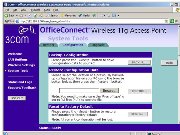
Select the *Configuration* tab to display the *Configuration* screen ([Figure 35](#)).
