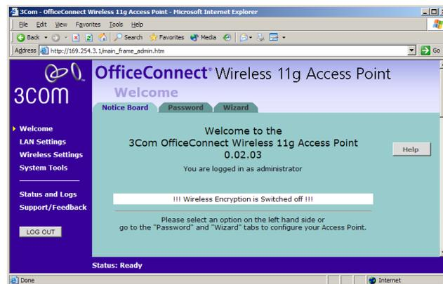
The *Welcome* section allows you to view the Notice board and to change your Password. You can also gain access to the Configuration Wizard. (See ["Accessing the Wizard"](#) on [page 21](#) for details).
