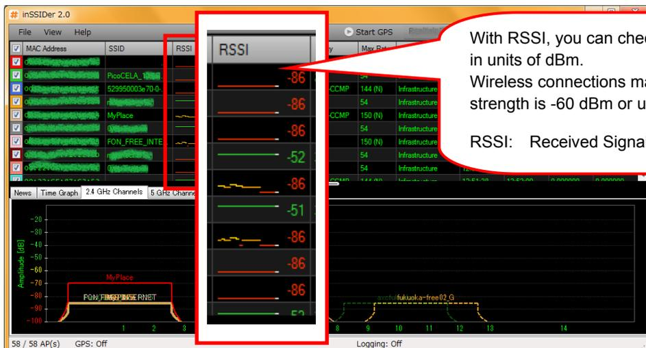
With RSSI, you can check the received signal strength in units of dBm.
