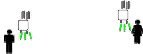
The LED flashes one to four times to indicate the strength of the link (more flashes mean a stronger link).
