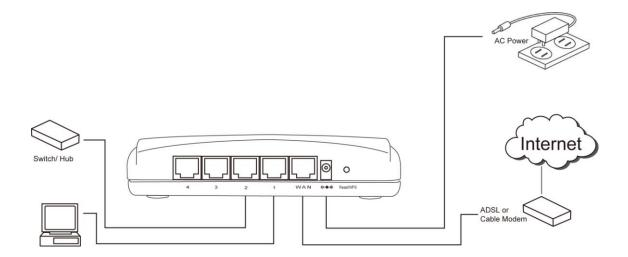
4. Please check all LEDs on the front panel. 'PWR' LED should be steadily on, WAN and LAN LEDs should be on if the computer / network device connected to the respective port of the router is powered on and correctly connected. If PWD LED is not on, or any LED you expected is not on, please recheck the cabling, or jump to '4-2 Troubleshooting' for possible reasons and solution.
