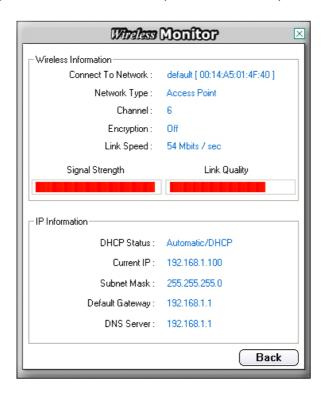
If you do not have adequate Signal Strength, try re-orienting the Access Point and/or the Wireless PCI Adapter to get a better reception.
