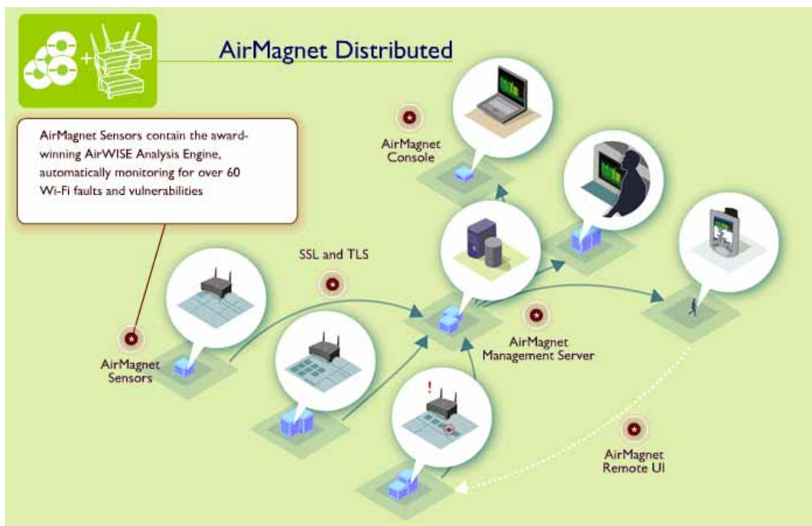
Figure 1: WLAN Network with AM-5020-11AG AirMagnet SmartEdge Sensors Installed AirMagnet Enterprise Console – provides the graphical user interface into the server from any
