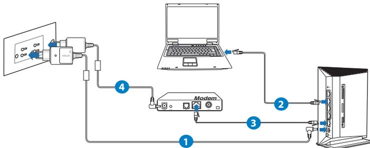
1. Insert your wireless router's AC adapter to the DC-In port and plug it to a power outlet.
