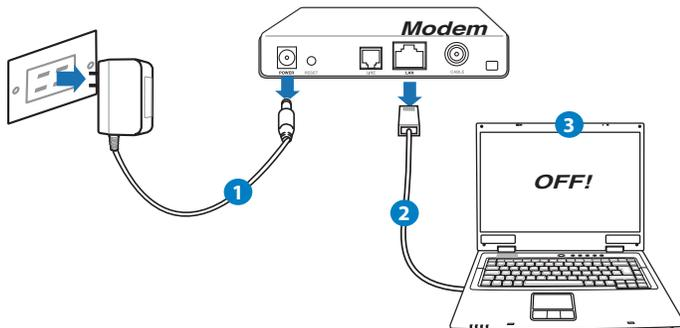
1. Unplug the AC adapter from the power outlet and disconnect it from your cable/ADSL modem.
