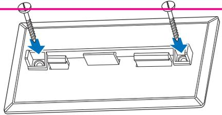
2. Locate the mounting holes at the back of the wireless router.
