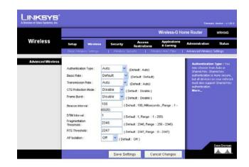
Figure 5-28: Wireless Tab - Advanced Wireless Settings
