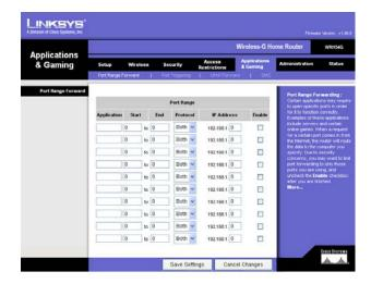
Figure 5-35: Applications and Gaming Tab - Port Range Forward
