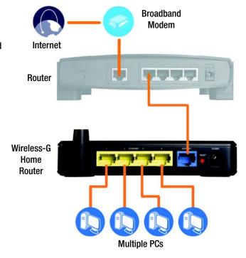
Figure 4-4: Diagram for Connection to Another Router
