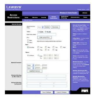
Figure 5-31: Access Restrictions Tab - Internet Access
