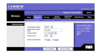
Figure 5-19: Wireless Tab - Basic Wireless Settings
