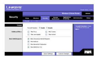
Figure 5-29: Security Tab - Firewall
