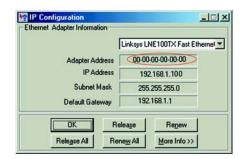
Figure E-2: MAC Address/Adapter Address
