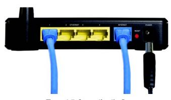
Figure 4-7: Connecting the Power
