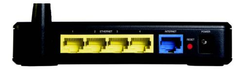
Figure 3-1: The Router's Back Panel
