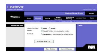
Figure 5-26: Wireless Tab - Wireless MAC Filter
