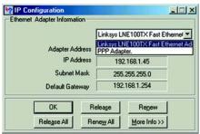
**Figure E-1: IP Configuration Screen**
