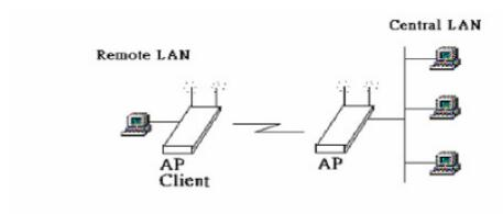
Wireless Bridge: The Wireless Bridge can communicate with any Wireless Bridge available in the same channel. When the Authorization Algorithm, is enabled, the Wireless Bridge can communicate with any Wireless Bridge whose BSSID exists.
