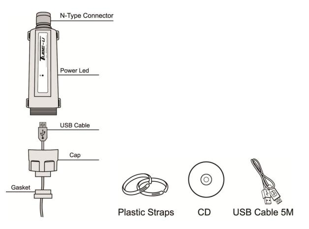
Use the plastic strap to secure your unit with a cylinder. Connect your 5M USB cable to the button of the unit.
