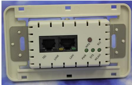
**Step 3 :** Line-up and push the Top faceplate onto Bottom faceplate until it snaps securely into place.
