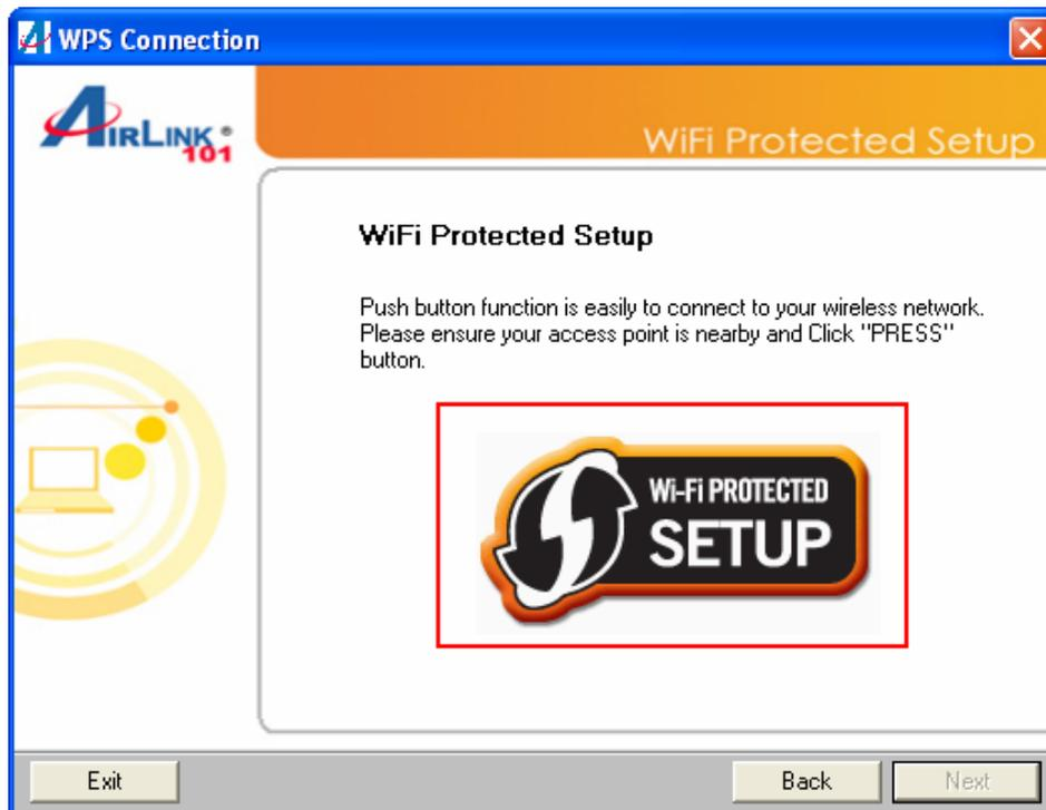
**Step 3b** Push the WPS button on the router, and the blue LED will start blinking. The router will now start the handshake with the wireless adapter, then the connection will be built up in couple minutes.
