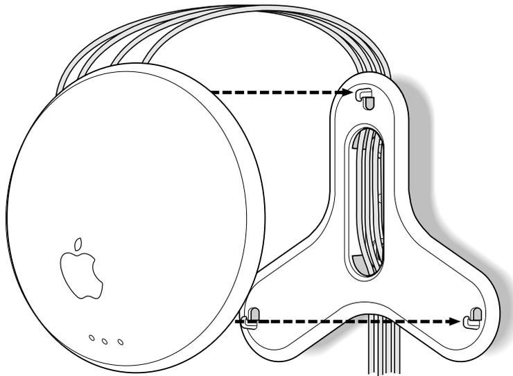
**Note:** The mounting bracket has enough space for four cables (power, phone, and two Ethernet cables), as shown in the illustration. In most cases only two cables are used.
