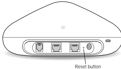
The middle light flashes green, indicating that the base station is in reset mode. The base station remains in reset mode for five minutes. If you do not make your changes within five minutes of pressing the reset button, you must reset it again.
