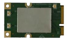
IEEE Dual Band 802.11n USB2.0 module for DTV
