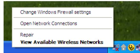
2. Highlight the wireless network (SSID) you would like to connect to and click **Connect**.
