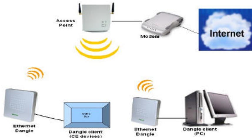
An Ethernet dangle is a device that connected to a client (e.g., PC, CE - Consumer Electronics devices) with one to one with Ethernet. The Ethernet dangle uses the MAC address of the dangle client / PC to communicate with remote 2.4/5 GHz wireless device (complied with IEEE 802.11a/b/g). The Ethernet dangle let your PC or CE (Game box, Set-top box) devices communicates with wireless access point device that extent your existing home/CE entertainment network to surf the Internet.
