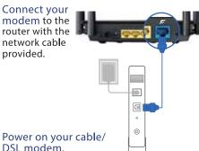
Check your cable/DSL modem LED lights to ensure the connection is active.
