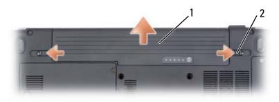
1 battery 2 battery release latches (2)
