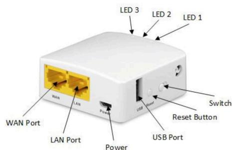
Power to the GLI Mini Router is provided by connect the power lead (supplied) to the power adaptor (buy separately) and then to the power interface on the GLI Mini Router.
