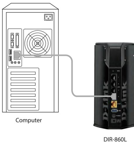
4. Plug one end of the included Ethernet cable that came with your router into the yellow port labeled INTERNET on the back of the router. Plug the other end of this cable into the Ethernet port on your modem.
