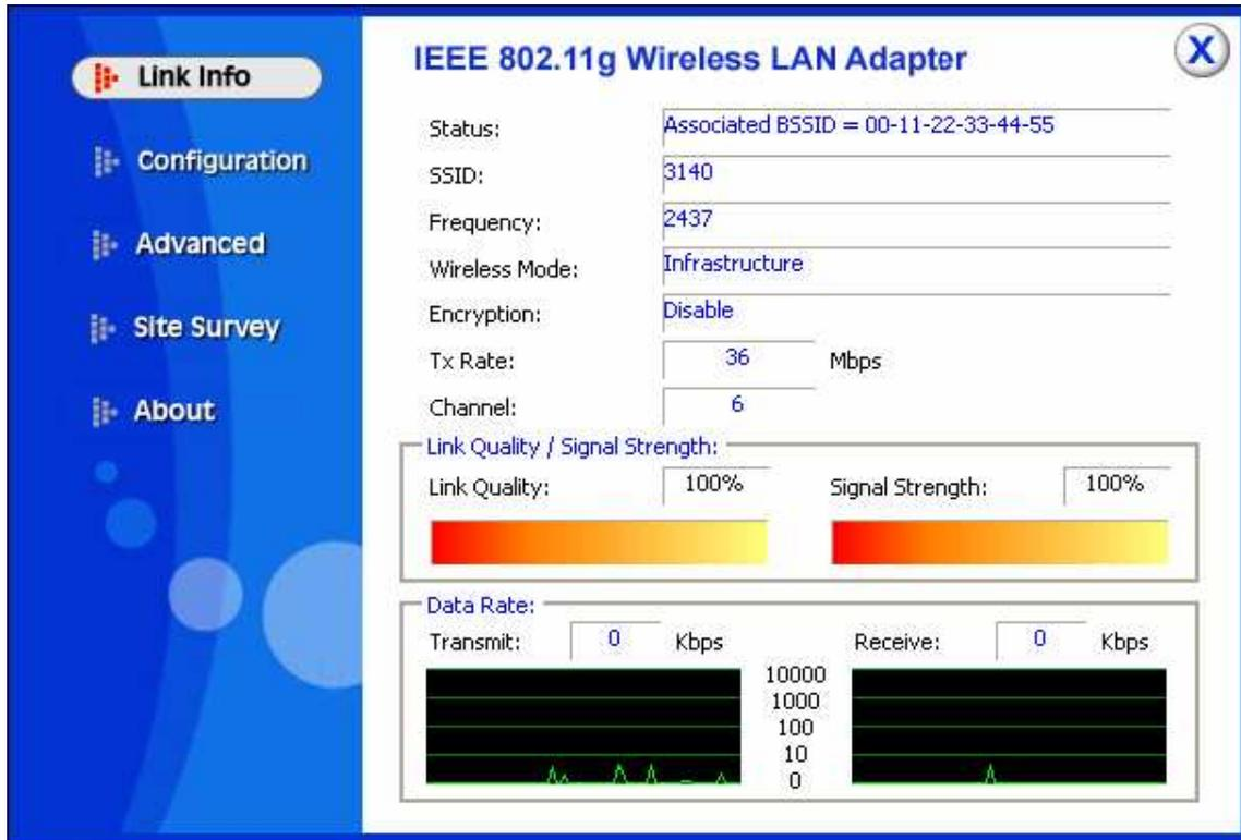
**Status:** Shows the associated BSSID, which can be used to identify the wireless network.
