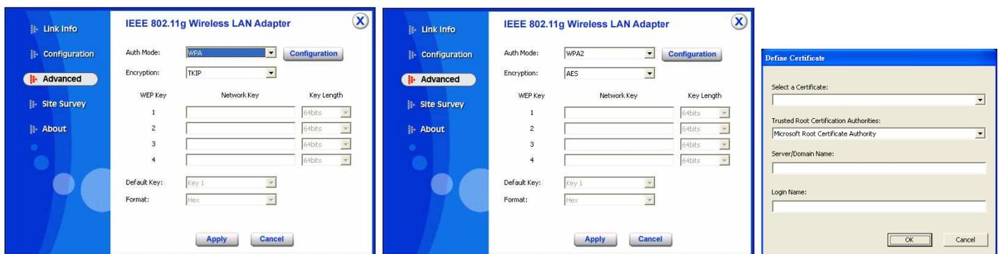
If WPA or WPA2 is selected, the above screen is shown. Please select the encryption type from drop down menu and press **Configuration** button to configure parameters for the RADIUS server.
