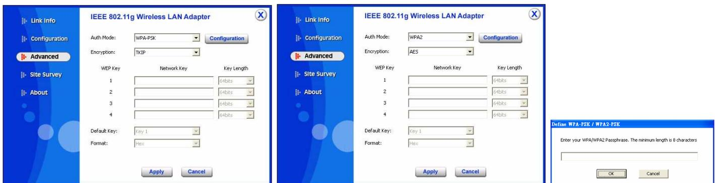
If WPA-PSK or WPA2-PSK is selected, the above screen is shown. Please select the encryption type from drop down menu and press **Configuration** button to configure the passphrase key.
