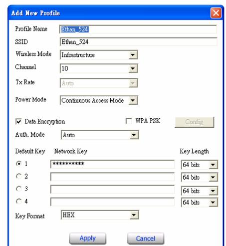
**Add:** Adds a profile. Then, the following screen would appear. User can enter the necessary information required for accessing Access Points or Wireless Router.
