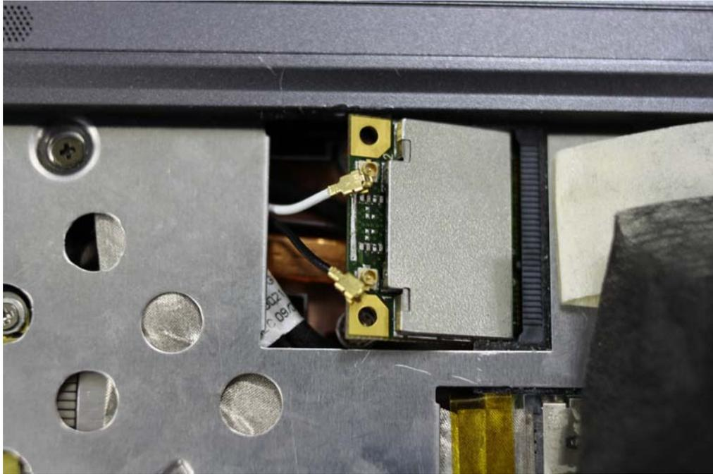
Step 3. Connect two external Wi-Fi antennas on I-PEX connectors.
