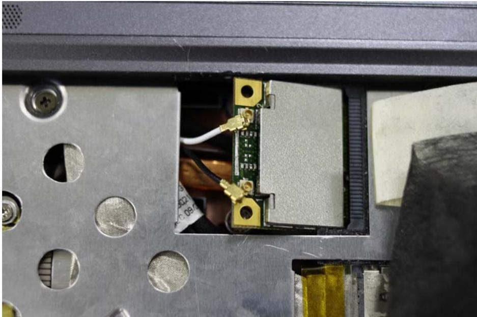
Step 3. Remove the Wireless PCIe MiniCard module board from PCIe MiniCard connector port.
