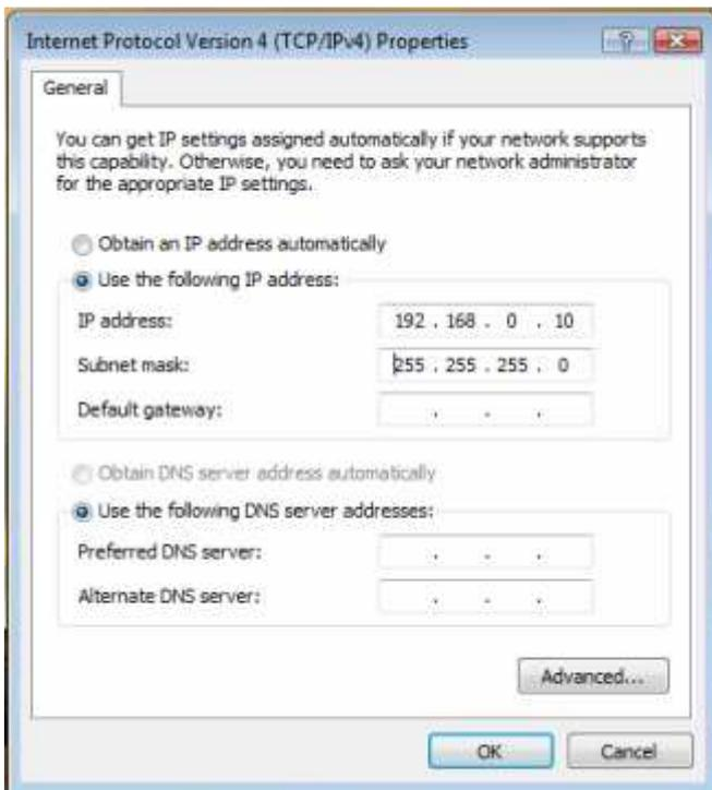
\*Note: the IP address of the other wireless card should be set with the same subnet mask
