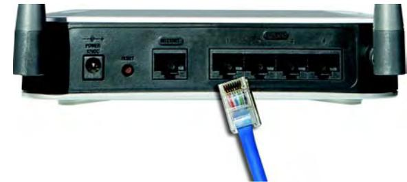
**Figure 5-1: Connect to LAN Ports**
