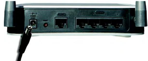
**Figure 5-5: Connect to Power Port**
