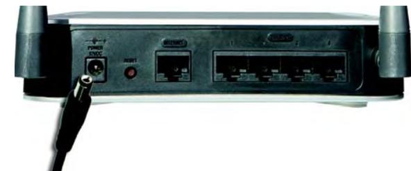
**Figure 5-3: Connect to Power Port**
