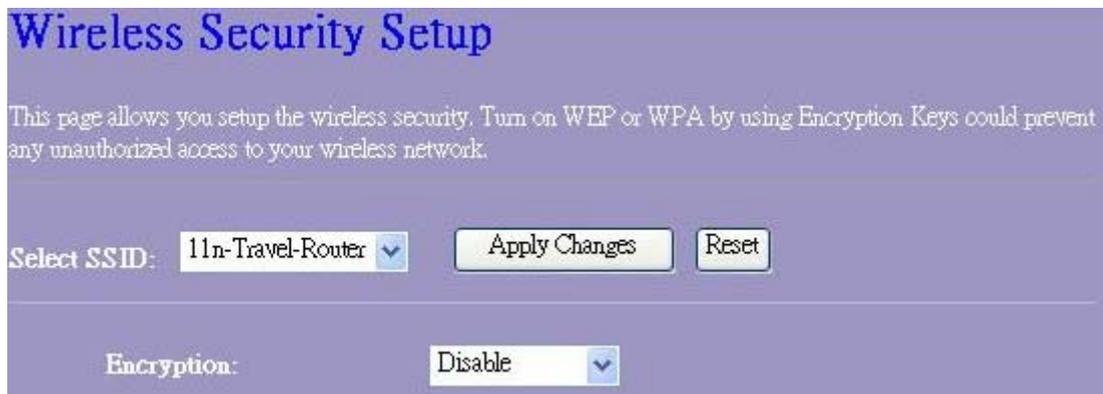
The screenshot shows the 'Wireless Security Setup' page. At the top, it says 'This page allows you setup the wireless security. Turn on WEP or WPA by using Encryption Keys could prevent any unauthorized access to your wireless network.' Below this, there is a 'Select SSID:' dropdown menu with '11n-Travel-Router' selected. To the right of the dropdown are two buttons: 'Apply Changes' and 'Reset'. Below the SSID dropdown, there is an 'Encryption:' dropdown menu with 'Disable' selected.
