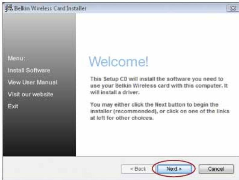
**Note:** If the Belkin Wireless Card Installer screen does not appear within 20 seconds, access your CD-ROM by double-clicking on the “My Computer” icon; then double-click on the CD-ROM drive into which the installation CD has been placed. If the Installer does not start automatically, double-click on the icon named “Installer.exe”.
