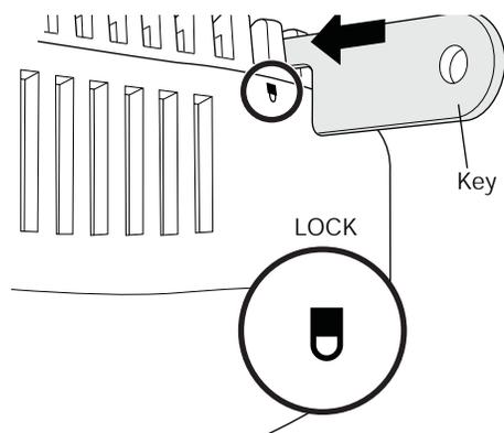
4. Insert the locking key and apply a small suitcase lock as shown in [Figure 41](#).
