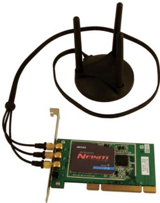
The WLI-PCI-G300N comes with a dedicated antenna module with three diversity antennas. This antenna module is designed for use with the WLI-PCI-G300N only. Do not use the WLI-PCI-G300N's antenna module with any other wireless product, and don't use any other antennas with the WLI-PCI-G300N. They are designed to work together.
