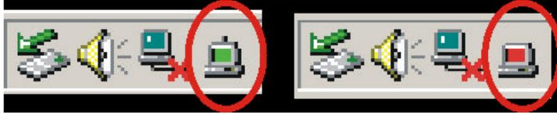
When the icon in the toolbar represents in green color, it is properly connected to the network and if it represents in red color, then it is not connected to the network.
