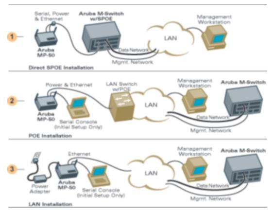
The Aruba 50 can be installed in your network using the following topologies:
