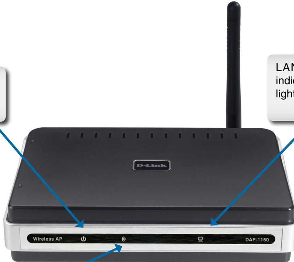
**WLAN:** Blinking green light indicates wireless activity; solid green light indicates connection
